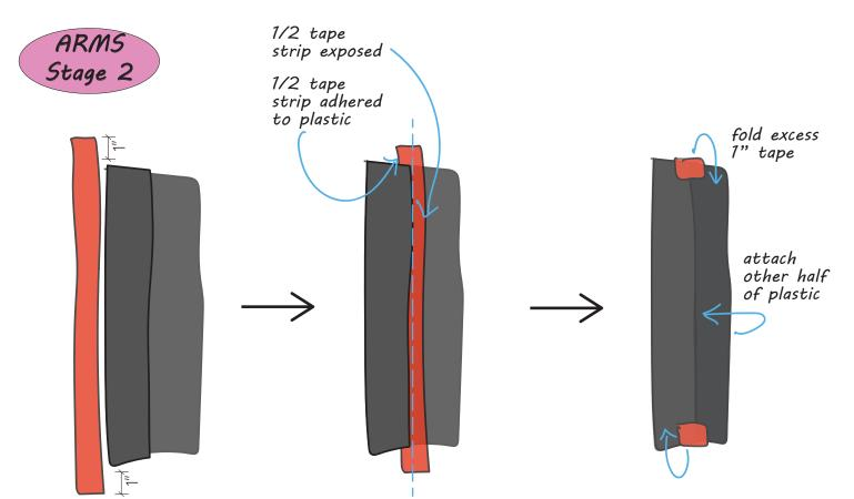
Cut a piece of duct tape to excess the plastic sleeve by 1 inch each side.
