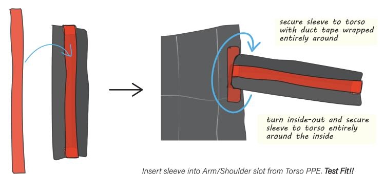
Take a second strip of duct tape same length as before and secure and close the outside seam.
